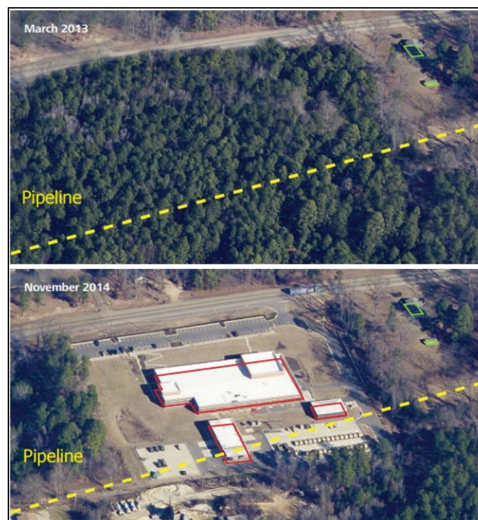
Figure 3. Airborne data collection alerting a utility company that there is a warehouse in the impact area of the gas pipeline. (Brown, 2012)
