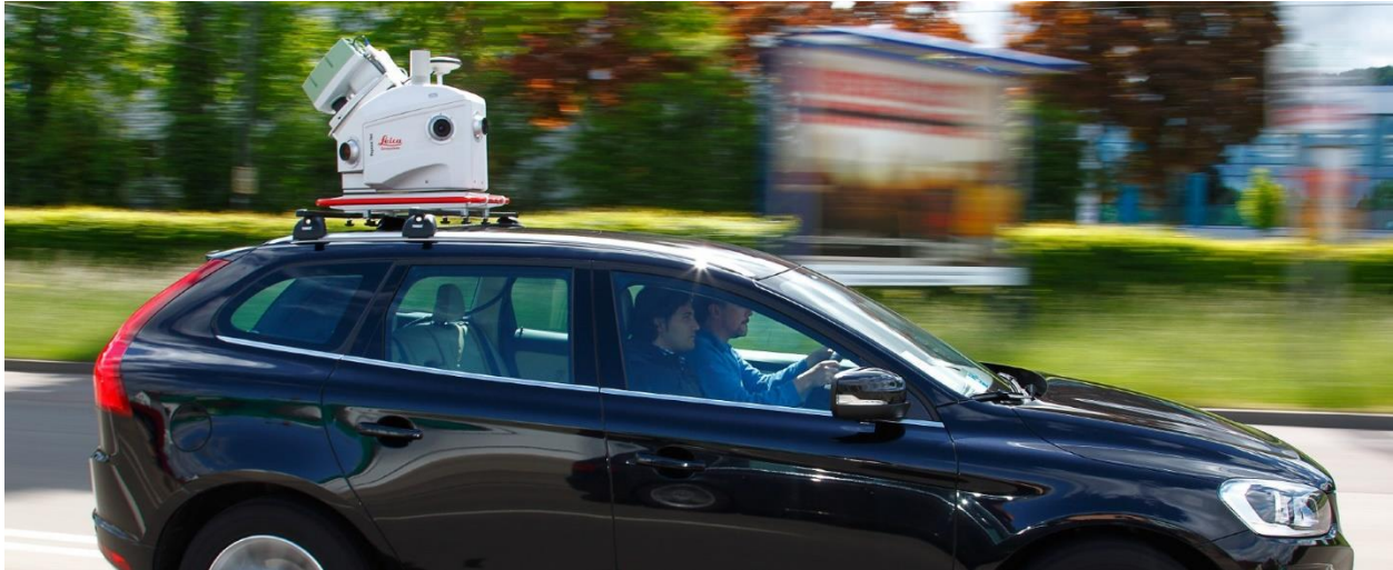
Figure 2: Pegasus 2 platform by Leica Geosystems mounted on a vehicle. (Source: Leica Geosystems)
