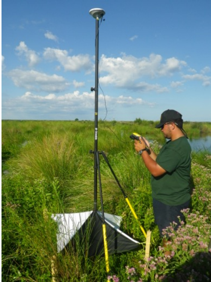
Figure 6: GPS Survey of a ground control point.
