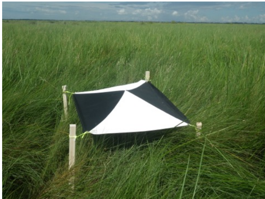
Figure 5: Example of a ground control point photo target.
