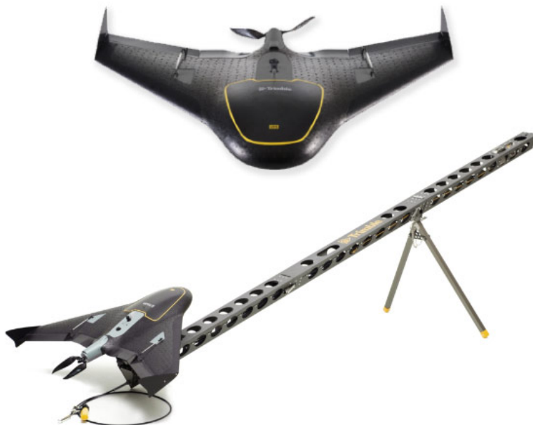
Figure 7: Trimble UX5 aerial imaging rover used in this project.
