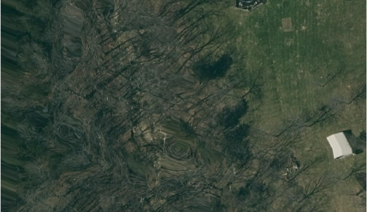
Appendix 2. Example of Smearing and Warping in Orthoimagery Pixels Encountered During Testing with Unfiltered Phodar
