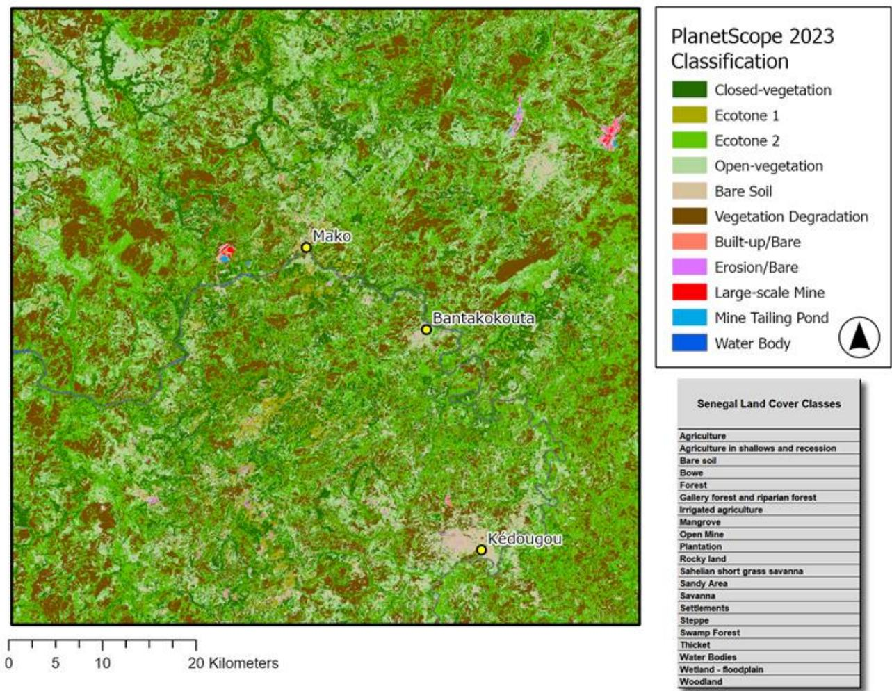
Figure 34. PlanetScope (4.77 meters) classified in eCognition using unsupervised classification and the multi-threshold segmentation. The results demonstrate that more detail can mean more vegetation classifications.
