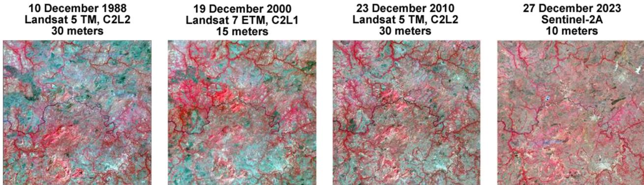
Figure 7. The primary satellite imagery was used to set the resolution for each eCognition project. Landsat 7 ETM and Landsat 5 TM used B4, B3, B2 , and Sentinel 2A used B8, B4, B3 (RGB) to display healthy vegetation in infrared.
