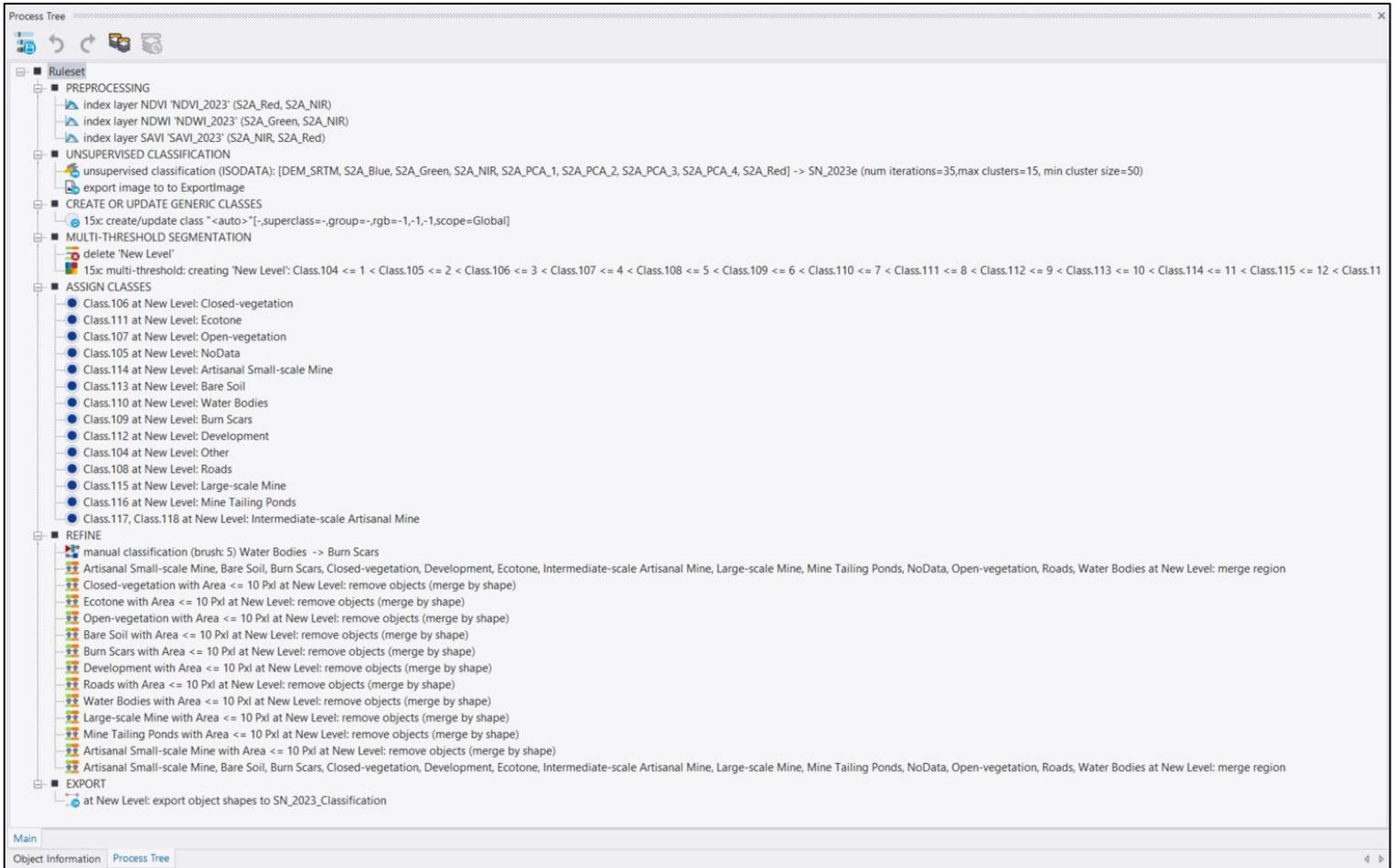
3. In PREPROCESSING you build canned indices within eCognition. You would first **Insert Child Process** and then search for the algorithm **index layer calculation**. There is a drop-down window to select from nine different indices.
