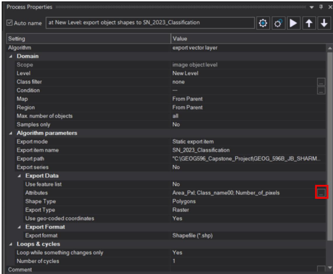
15. Click on the drop-down menu in **Attributes**, and the **Edit Attribute Table Columns** window will open. At the bottom, click on the **Add/Remove Features** button to open the **Select Multiple Features** window as pictured below.
