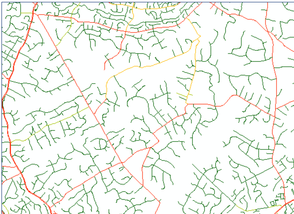
Figure 5. An example of the barriers represented by LTS 3–4 roads (yellow and red); none of these neighborhoods can connect to one another.
