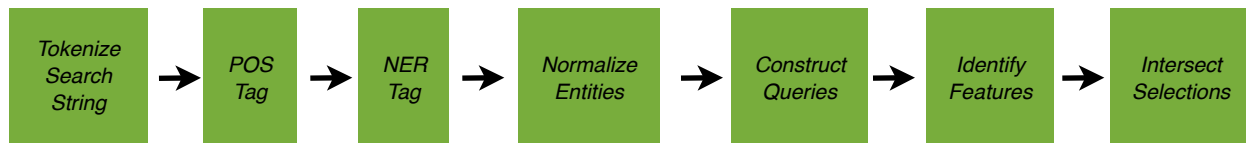
Figure 11 - NLP Search Application Query Processing Pipeline
