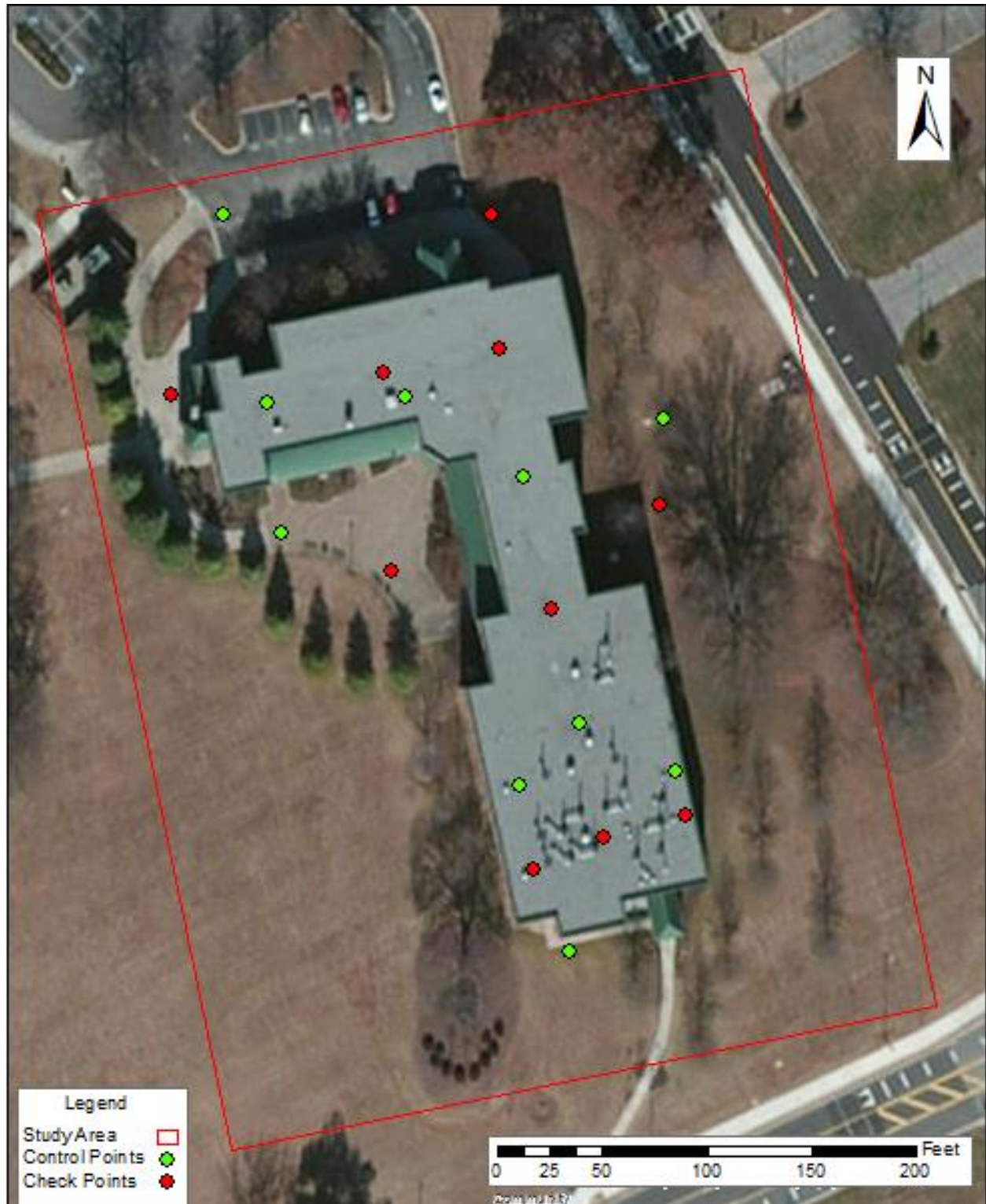
Figure 7. Locations of control points and check points that were collected for this project.
