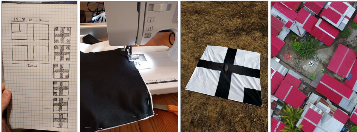
From left to right: sketching my designs, sewing, a ground control point as seen from the ground with a Garmin GPS device laid at the center, and a ground control point visible in imagery taken in the Philippines.
