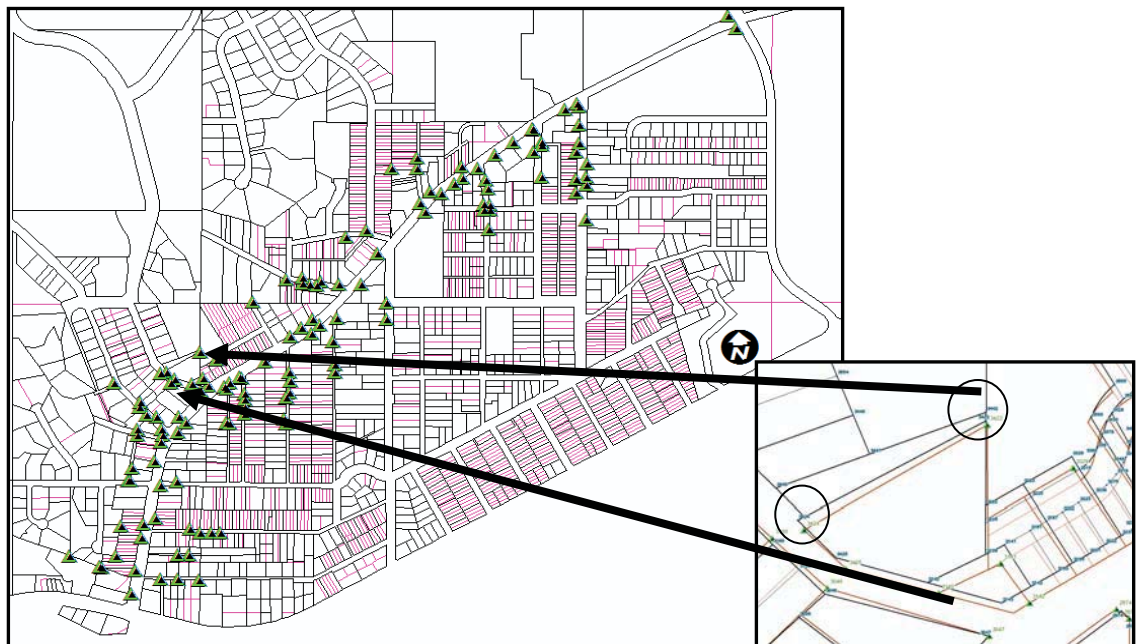
Figure 10. Control points loaded into the fabric for the study area and associated with the appropriate parcel corners.
