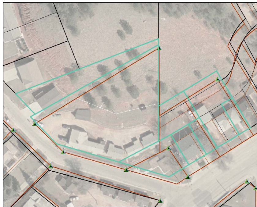
Figure 12. An example of an area of parcels that is well-balanced geometrically with evenly distributed control.
