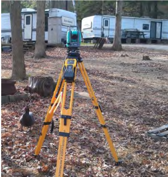
Figure 17: Surveyor’s total station and data collector placed over control point in MWCD campground. Photo by Author.
