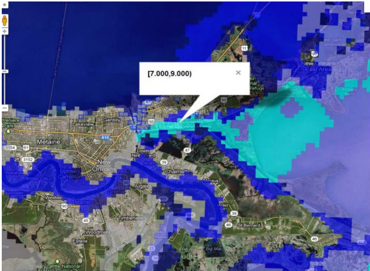
Figure 10 – Output from PHISH in the New Orleans area. Values in the balloon box indicate the range in feet between which the storm tide is forecasted to reach in the corresponding grid cell (Gibbs 2013).
