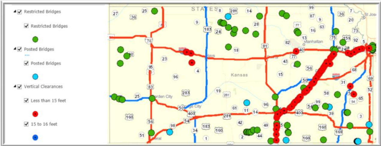
Figure 2.3. Load Posted, Load Restricted or Vertical Clearance Limited Bridges
