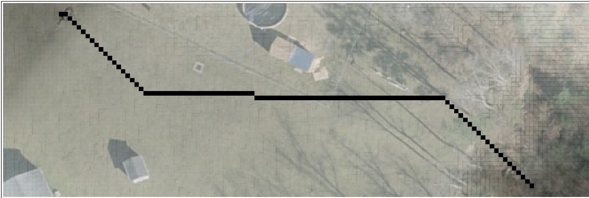
Image P: Crooked drainage path from an inlet (top left) to a forested gully (bottom right). Notice the drainage grate partway between the path endpoints. [Local data from the County of Prince George, VA . Imagery courtesy of the Commonwealth of Virginia . Terrain data from USGS.]
