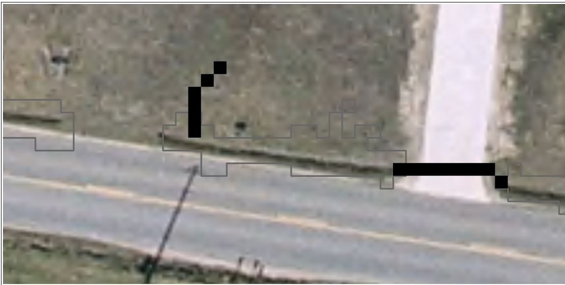
Image O: Chain of shallow sinks, representing a minor, roadside drainage path. The right path correctly connects under the driveway, but the left misses the other pipe and paths back into the yard. [Local data from the County of Prince George, VA . Imagery courtesy of the Commonwealth of Virginia .]
