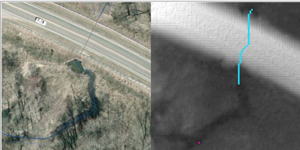
Image N: Left: Apparent stream path compared to aerial imagery and photogrammetric lines. Right: Drain path against terrain data, with the lowest sink cell highlighted. [Local data from the County of Prince George, VA . Imagery courtesy of the Commonwealth of Virginia . Terrain data from USGS.]
