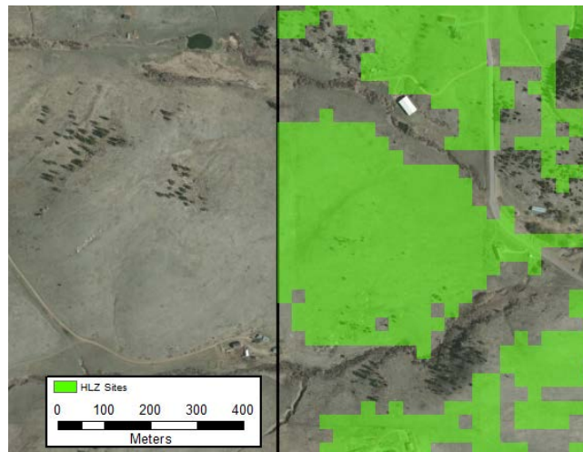
Figure 25: Edge Effect Limiting the Size of a Suitable Landing Zone. Background Image from ESRI Online – World Imagery (Environmental Systems Research Institute, 2013b)
