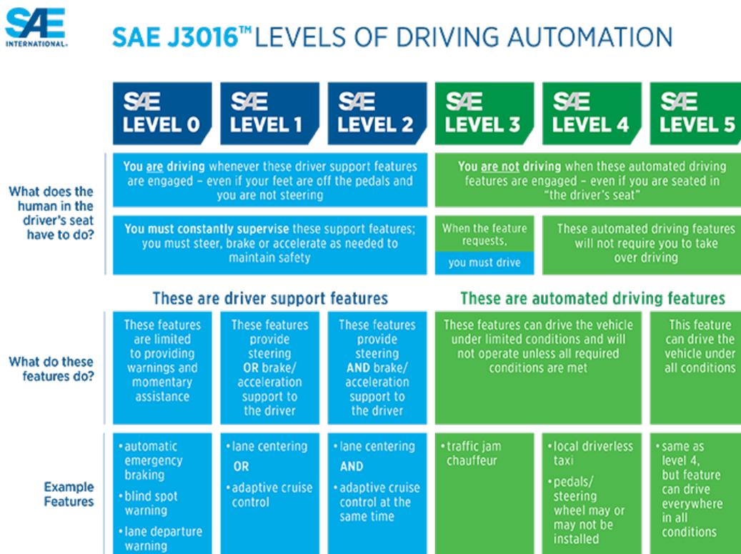
**Figure 1.** SAE Levels of Driving Automation (SAE International, 2018b): Levels 0-3 have automation features currently available for the public in various models while levels 4-5 are not available to the public.
