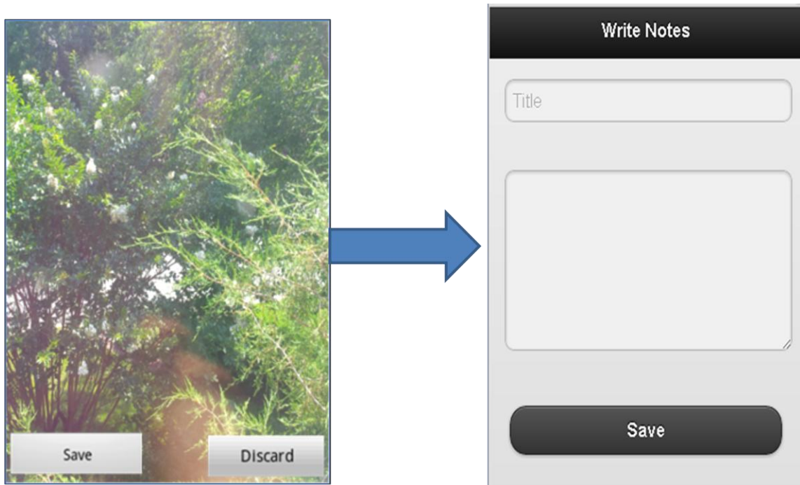
Figure 8: Once you tap on the image's Save button, the image is to be save to the phone's default camera storage folder and the "Write Notes" screen will pop-up for entering associated metadata. The Save button on Write Notes will save the new record of image's file path and metadata to the PhotoVideoNotes table.
