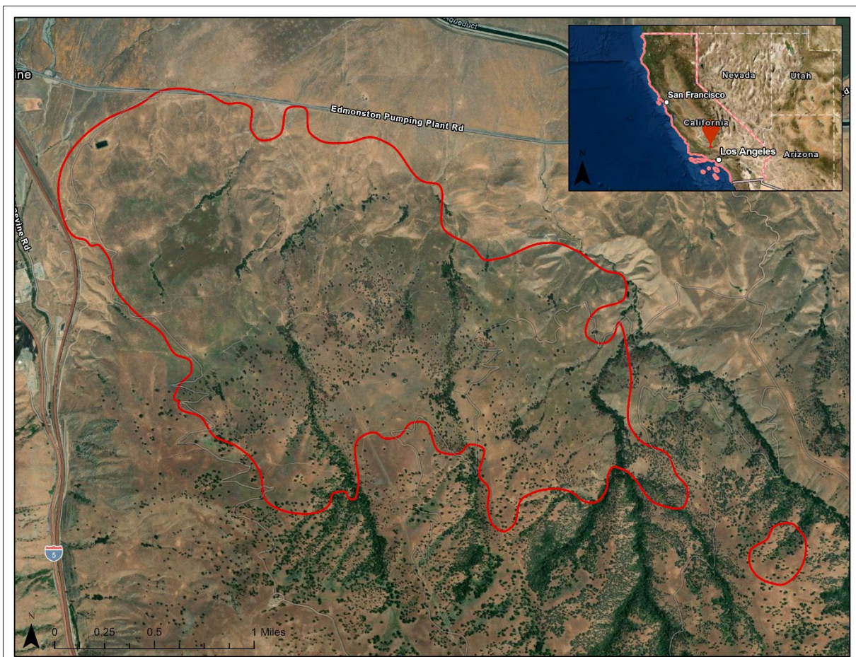
Figure 25. Results of the raster calculator operation to calculate the difference between the pre- and post-fire Landsat8 imagery and subsequent reclassification of pixel values to display a binary burn (pixel value 1) or unburned (pixel value 0) image. Red pixels represent burn areas while green represent unburned.
