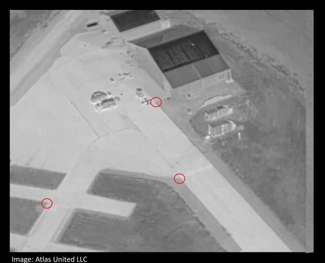
Plot photo-identifiable checkpoints in successive frames of motion imagery, then calculate NMAS CE90 statistics.
