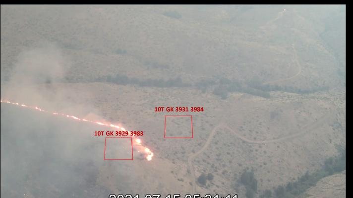
2021.07.15 05:31:11 GPS(40.0718,-120.1931,0.0M) BAROMETER:385.0M Identify a stratified random sample of heat and non-heat grid squares in processed dataset. Back-project each grid square to video, edit clips together, and disseminate to accuracy assessors for visual interpretation.
