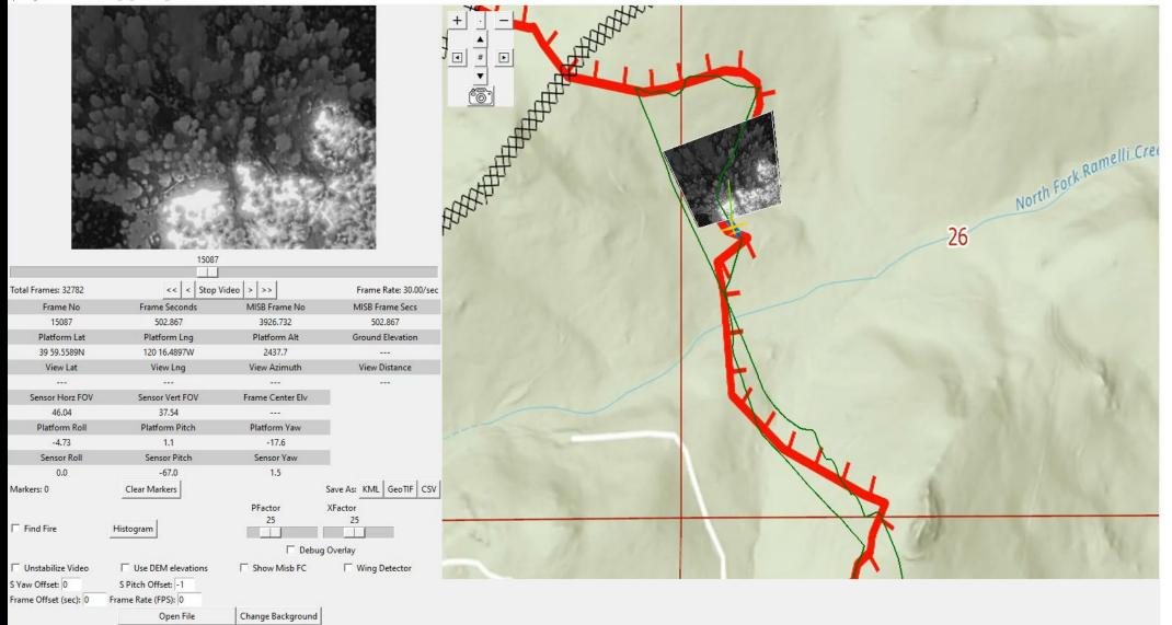
We use aircraft and sensor telemetry metadata, combined with elevation data, in order to georeferenced and terrain correct each video frame.
