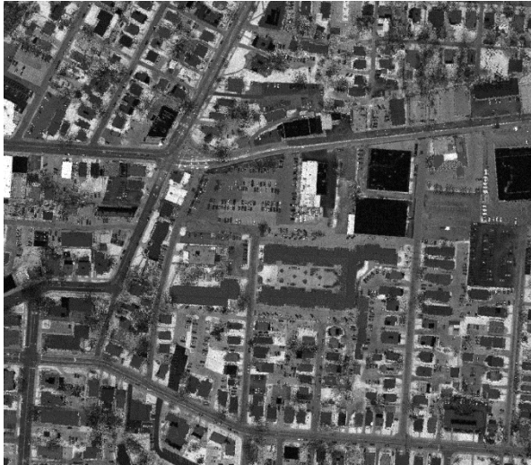
Figure 2 Example of lidar intensity raster showing a portion of downtown Athens, OH, filtered by ground and last of many returns. Bright values represent ground vegetation; darker values indicate paved surfaces. Dark pixel groupings shaped like trees are last of many returns. Light is absorbed when it passes through trees, resulting in a darker value.
