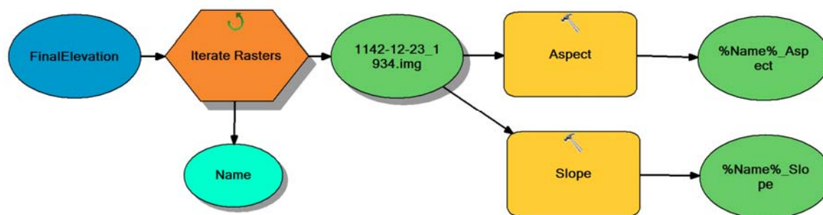
Figure 4. ArcGIS Modelbuilder model used to generate aspect and slope raster from each DEM
