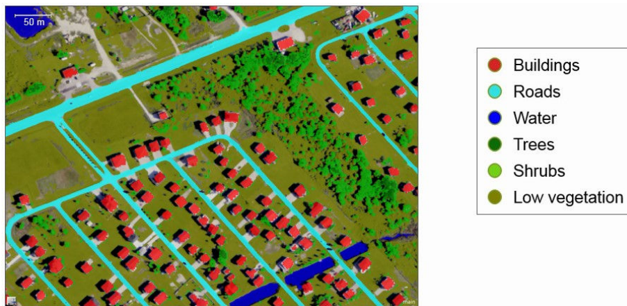
Figure 1: The image shows the OBIA classification of the six object types indicated in the legend. Classified objects are overlaid on a high resolution aerial image.
