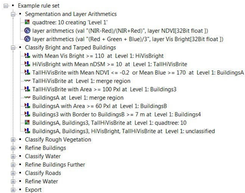
Figure 2: Example rule set showing the sequence of rules used to segment and classify objects.
