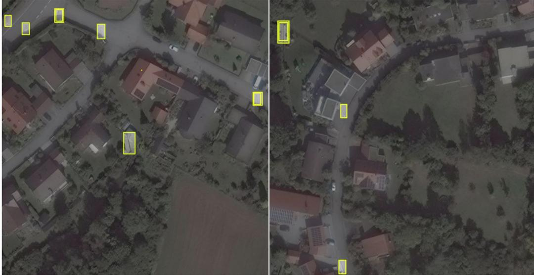
*Figure 9 illustrates example images from the final training session. In the **left** image the model produced 5 true positives and one false positive, correctly predicting the presence of electric poles 5 of 6 times. In the **right** image, the model produced 3 false positives, incorrectly predicting the presence of electric poles 3 of 3 times.*
