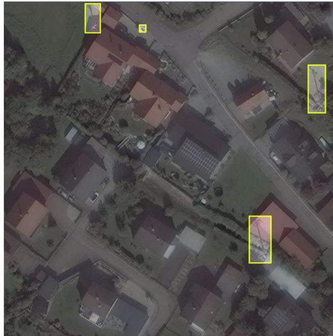
*Figure 2 shows the process of labeling electrical distribution structures in the acquired satellite imagery.*
