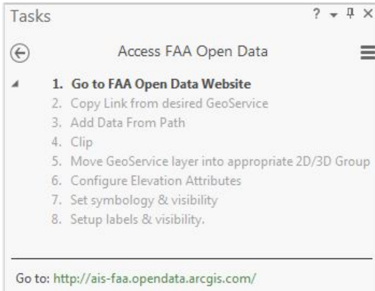
Figure 24. ArcGIS Tasks facilitate import and processing procedures for ZDV-3D data. Created in ArcGIS Pro (Esri, 2018).
