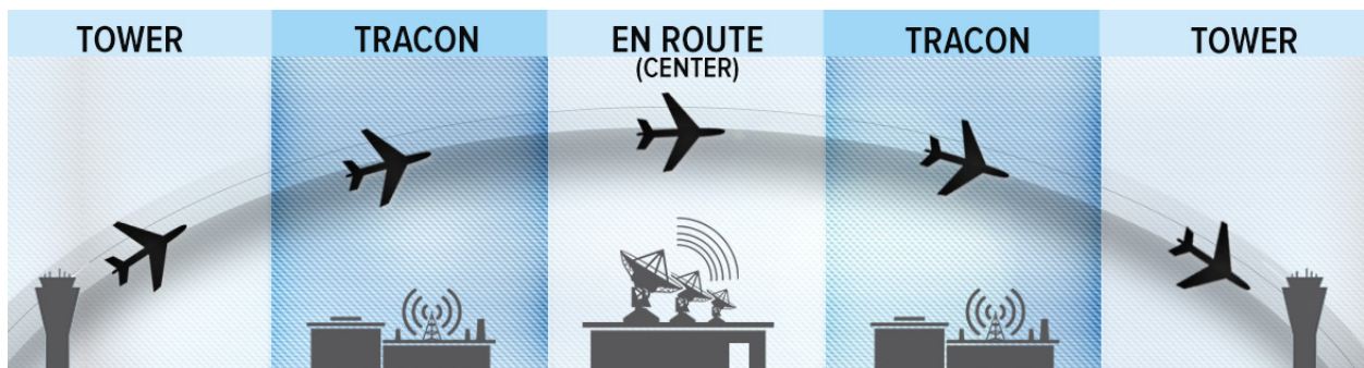
Figure 1. FAA En Route Traffic Control Centers role compared to Towers and TRACONs (Aviation Stack Exchange, 2016).
