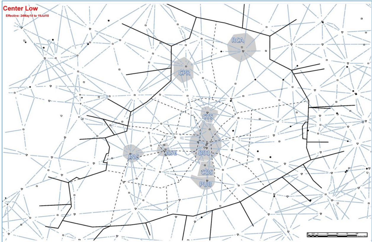
Figure 5. ZDV low altitude structure. Approach airspace is shaded gray, low altitude airways are blue, and sectors are black-dashed lines. Created in ArcGIS Desktop (Esri, 2017).
