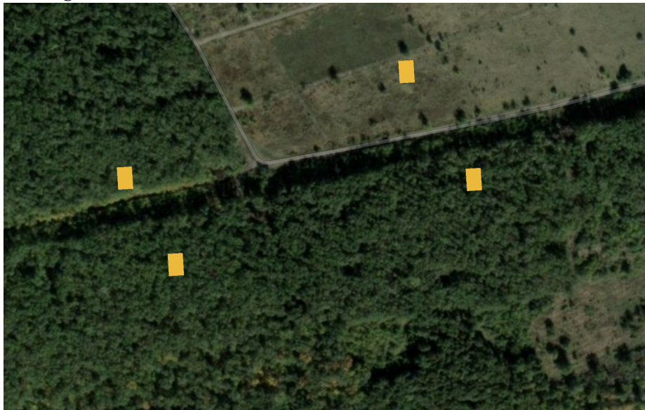
Fig. 9 Misclassified pixels in Donetsk forest and farm land, falsely identified as potential building damage
