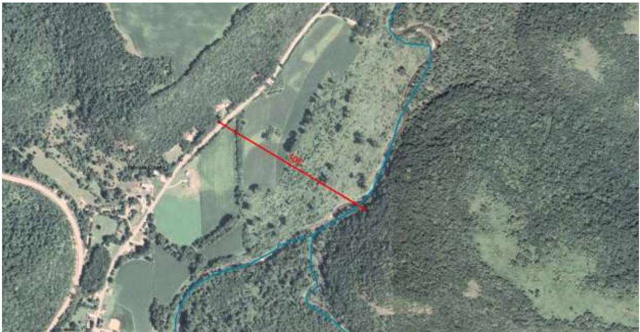
X Section Range 10C Whitewater Main branch. 0+00 is located right down stream on the SE end of the line and goes to the NW
