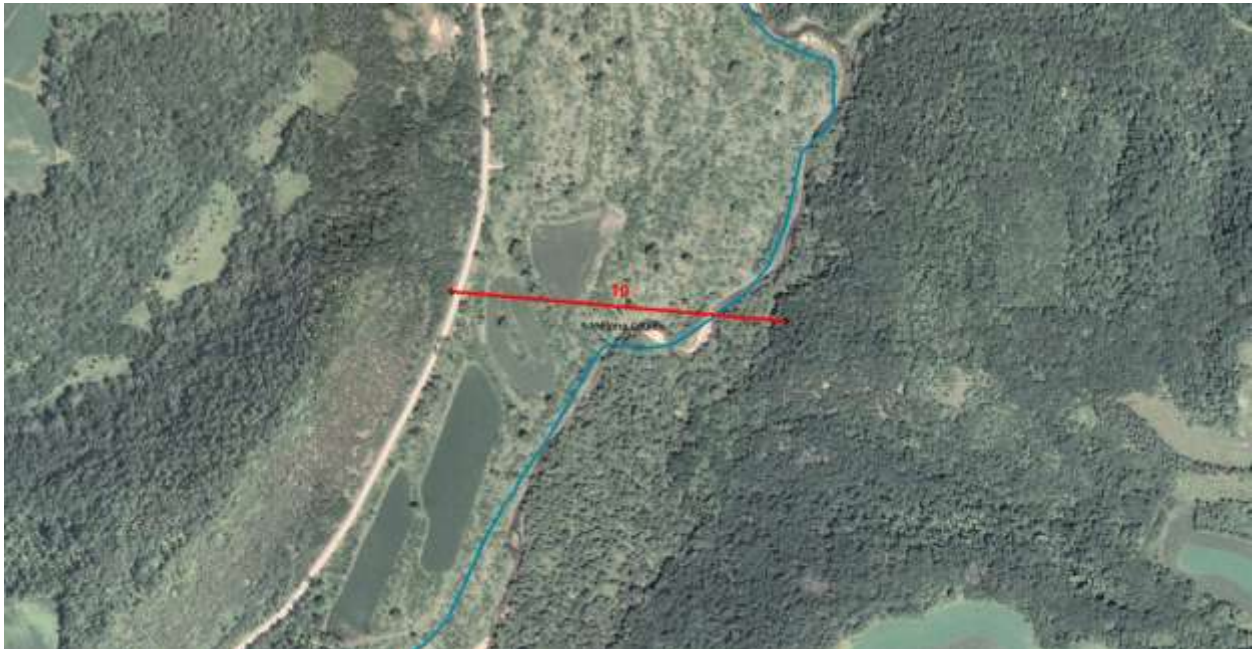
X Section Range 10 Whitewater Main branch. 0+00 is located right down stream and goes from east to west.
