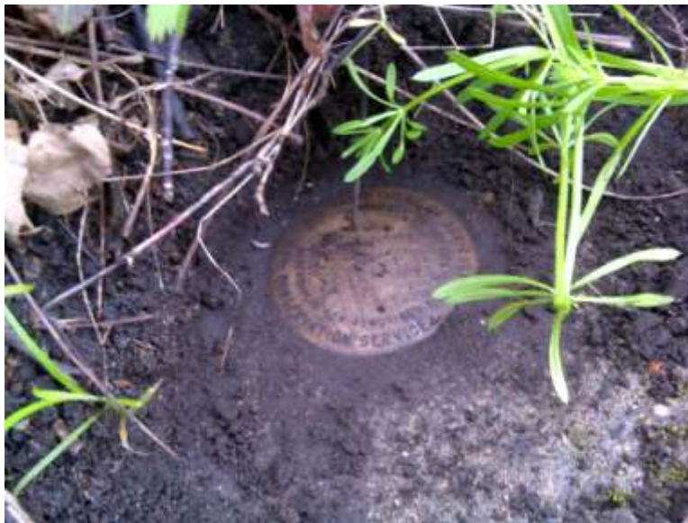
Monument 11B-S. Located 5/12/11. 11B-S is the only endpoint monument which is marked with a brass cap set in concrete. 11B-S could not be located during the 64 and 94 surveys and was considered lost until located by this study in the summer of 2011. Because the cap is brass the normal use of a metal detector did not work. The red point on the photo above was the assumed located location for many years. It was finally locate by running a line from 11B-N through a stake that was still in place on the earthen dike from the 94 survey. Measuring the surveyed distance from the notes and using the azimuth we got to within 5 feet of this location. A 4 foot steel rebar was driven into the ground next to the brass cap to aid in future locating. The beginning point 0+00 of Range 11B. Photo by author
