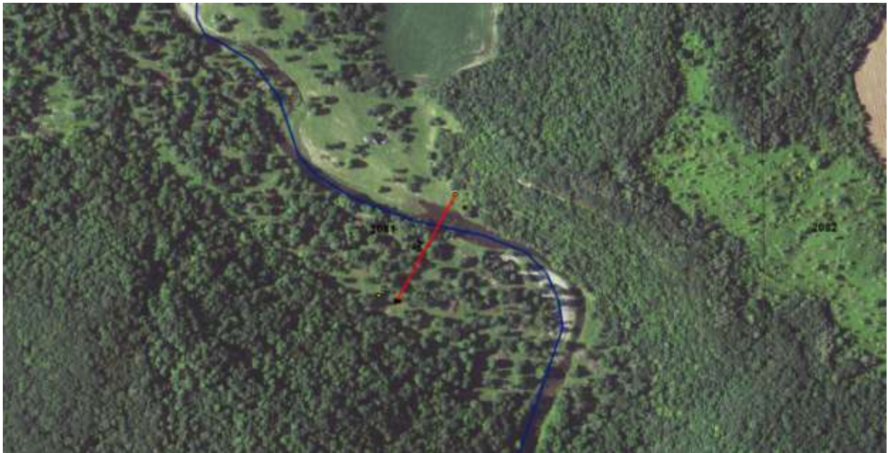
X Section Range SF-4 South Fork of the Whitewater River. 0+00 is located right down stream and is on the northeast end of the line.
