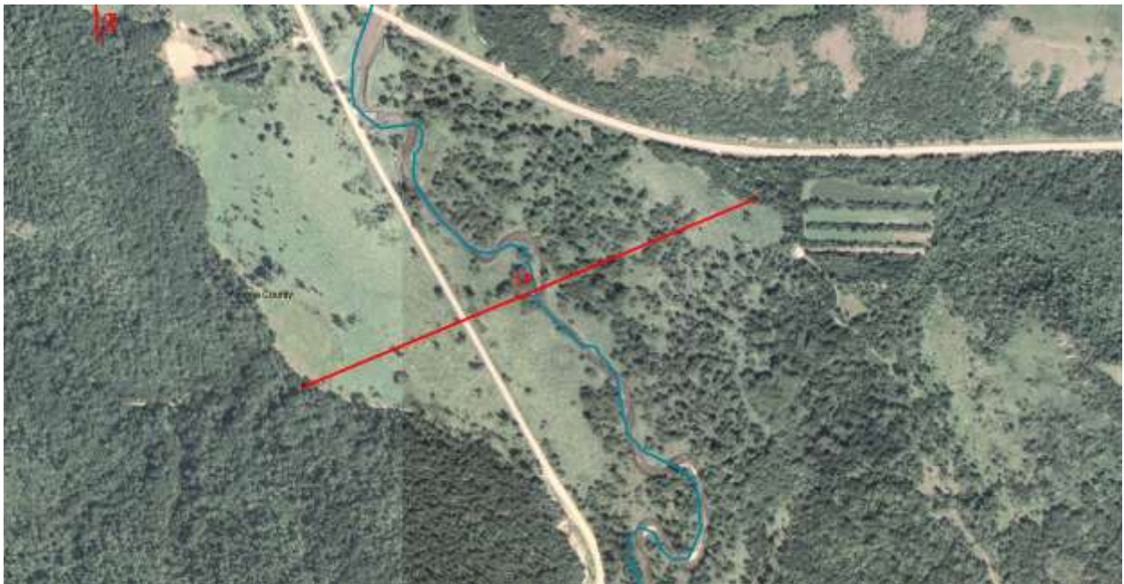
X Section Range 7A Whitewater Main branch. 0+00 is located right down stream and goes from northeast to southwest.
