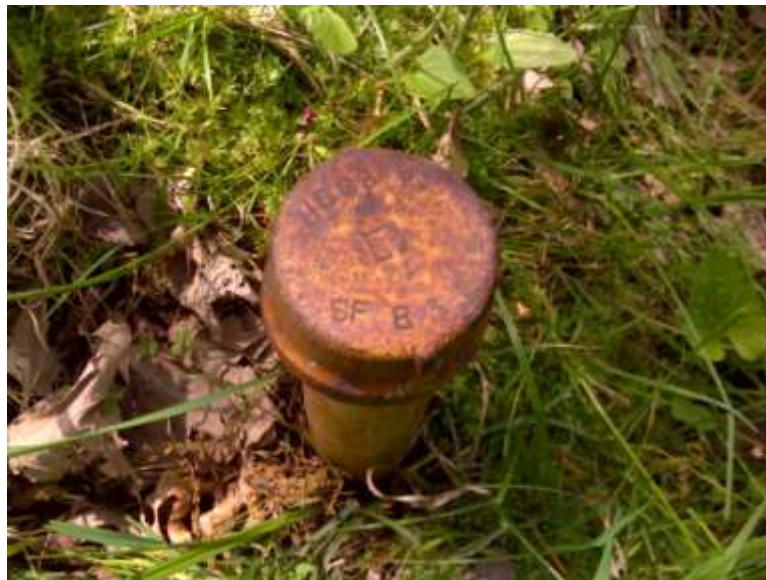
Monument S-3-L. Located 6/2/11. Located in a pasture area with scattered trees. This is also an example of how most of the caps are stamped. In this example it is a close up photo of the cap stamped with USGS and SF R 3 L. Photo by author
